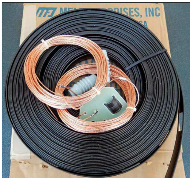
Figure 4 — The MFJ-1742 arrives preassembled with 100 feet of 450 \Omega ladder line.
