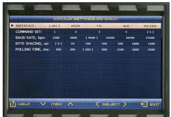
Figure 2 — The CAT/AUX screen is used to set up the transceiver interface so the amplifier will follow the transceiver's band changes automatically.
