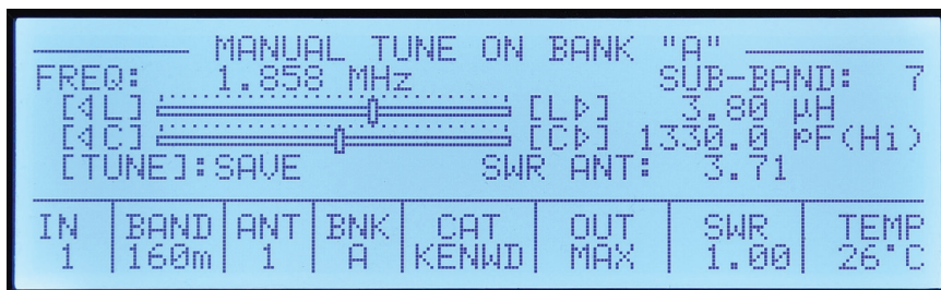
Figure 12 — The MANUAL TUNE screen allows adjustment of the inductance and capacitance values if the internal antenna tuner can't find a suitable match automatically. SWR is shown on both the antenna and amplifier sides of the ATU .
