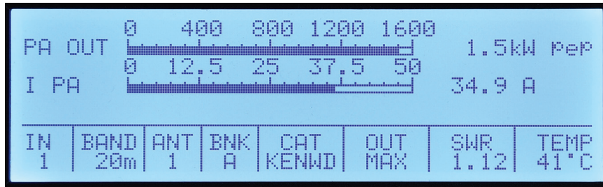
Figure 10 — Indicators along the bottom of the LCD show radio, band, antenna port, and selected bank, along with CAT (transceiver interface) setting, output level ( MAX , MID , LOW ), SWR on the amplifier side of the ATU, and temperature. The upper portion of the display shows RF output (both on a bar graph and as a numerical display) and PA current when the amplifier is ready to operate. A front-panel switch changes the upper display to PA voltage, indicators showing that the fans are running, and SWR on the antenna side of the tuner. In standby, the LCD shows exciter power (up to 200 W) and SWR on the antenna side of the ATU.
