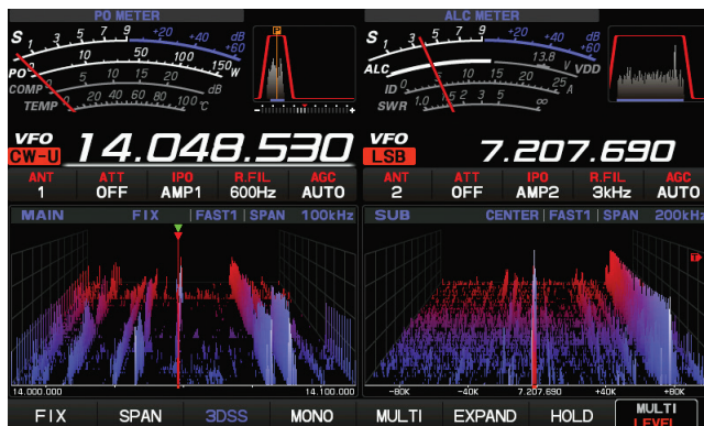
Figure 3 — Same as Figure 2, except a second spectrum view of the sub receiver display has been added to the right of the first spectrum display for the main receiver. Note that the second receiver is on a different band and using a different mode, bandwidth, and antenna. Either receiver can be tuned anywhere within the FTDX101D's tuning range, independent of the other receiver's settings. The two displays can also be one above the other, if you prefer — lots of flexibility available.
