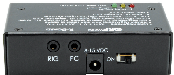
Figure 20 — Connections for the radio, computer, and power, plus an on/off switch, are located along the bottom of the K-Board. The SideKar is similar.
