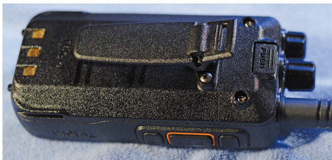
Figure 6 — The rear of the radio, showing the battery release button (right), plus the push-to-talk button (bottom, outlined in orange) and, on either side of it, the two dual-action programmable buttons. I have mine programmed for power-level toggling, squelch opening, and quick scanning.
