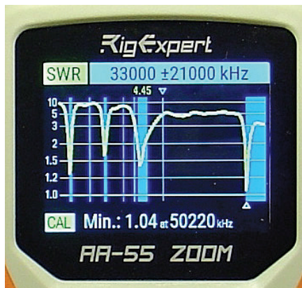
Figure 14 — A 10 – 60 MHz scan of the reviewer's TH-1 20/15/10/6 meter multiband dipole.
