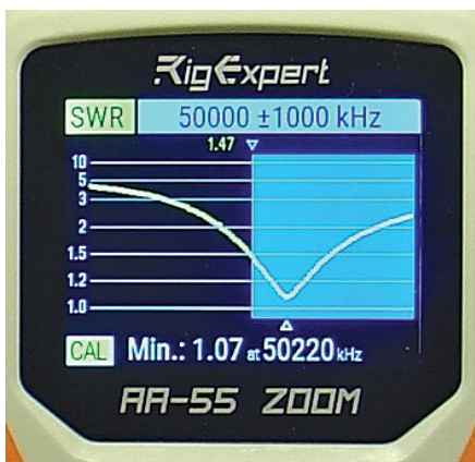
Figure 16 — A scan of the TH-1 multiband dipole, showing the response over the 6-meter band.
