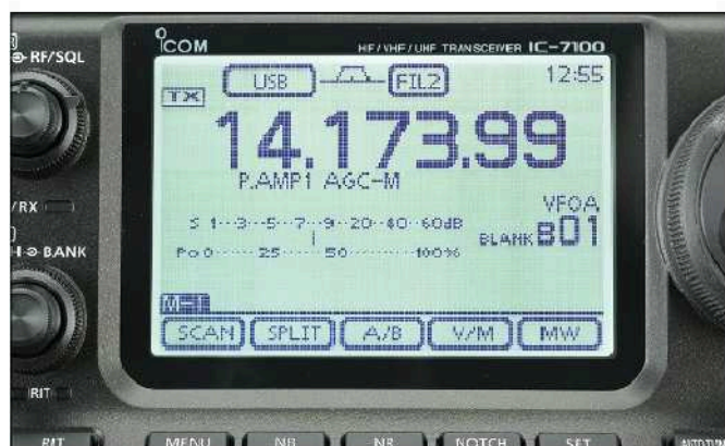
Figure 5 — The IC-7100's screen is larger than that on the IC-706 and IC-7000. Touching various spots on the screen such as the soft keys across the bottom or the frequency display brings up menus or changes settings.
