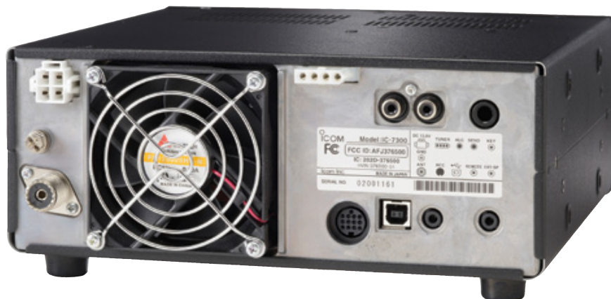
Figure 1 — The IC-7300’s rear panel has connections for a CW paddle for the internal keyer or external key/keyer; an external speaker; ALC and TR switching for an amplifier; remote control via the optional RS-BA1 software or an Icom CI-V device; a USB port for radio control and digital mode operation; an ACC socket for connecting a TNC or PC for digital modes, and a jack for connection to any of Icom’s accessory antenna tuners or tuned antennas.
