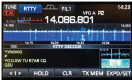
Figure 5 — The built-in RTTY decoder features a window on the lower right with a visual tuning aid — just line up the mark and space signals with the vertical bars. Up to four lines of decoded text are displayed at the lower left.
