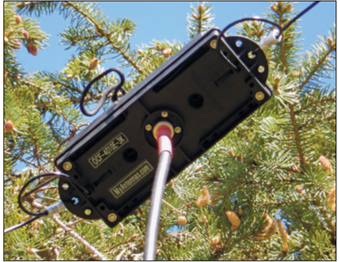
Figure 12 — The feed point with balun/center insulator installed at a height of 30 feet. The 53-foot leg extends horizontally while the 13-foot leg slopes downward.
