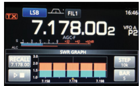
Figure 7 — The SWR graphing function offers a visual indication of antenna system SWR over an adjustable frequency range.
