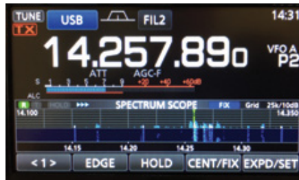
Figure 6 — The IC-7300's real-time spectrum scope shows both panadapter and waterfall displays. The frequency span is adjustable in several steps and can be set to show a fixed portion of the band or centered around the operating frequency.
