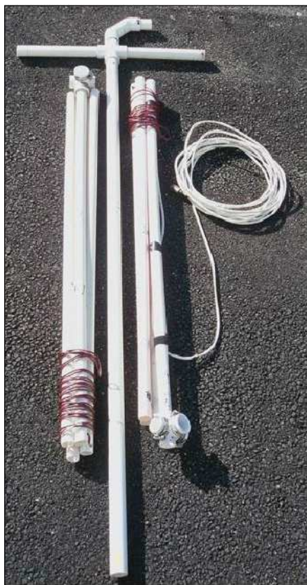
Figure 2 — Easy-to-stow disassembled antenna components.
