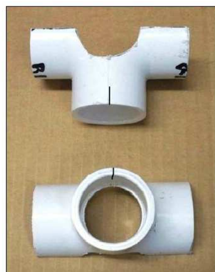
Figure 1 — Split a PVC T and file away material so that with a four-way PVC cross you have a fixture with five openings.
