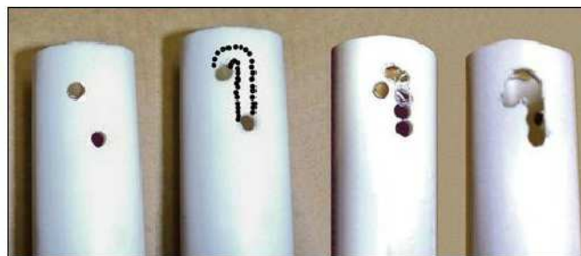
Figure 4 — Steps for making the J holes.
