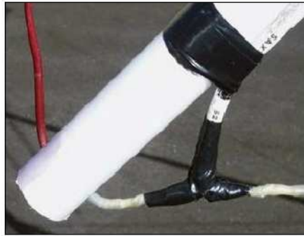
Figure 5 — Detail of the coax feed line connection.
