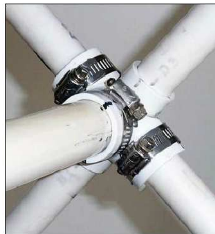
Figure 3 — The five-opening fixture ties the boom end to the four spreaders.
