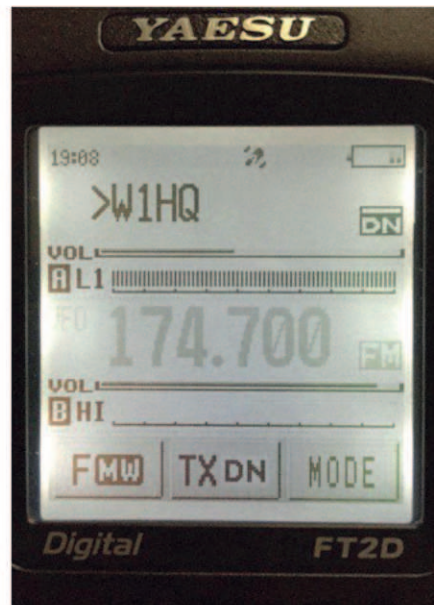
Figure 4 — Receiving a C4FM digital transmission from ARRL Headquarters station W1HQ on VFO A. The FT2DR was originally in analog FM mode, but it instantly switched to digital when it detected W1HQ’s digital signal. Notice the DN symbol at the upper right.
