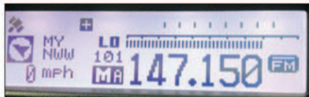
Figure 1 — During analog FM operation, the GPS display on the left-hand side shows your heading and speed.
