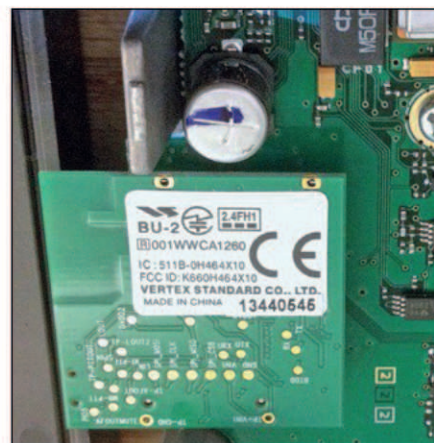
Figure 2 — The BU-2 Bluetooth adapter installed in the FTM-100DR. You must remove the top of the FTM-100DR case to plug it in.
