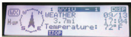
Figure 3 — When the FTM-100DR's TNC decodes an APRS beacon, the text and transmitting station's compass heading and distance are displayed.
